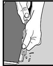
If necessary, place 12mm spacers between the last planks and the wall to keep the planks together during the curing time of the glue.
