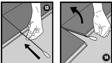
**Disassembling with Valinge Release Tool**
