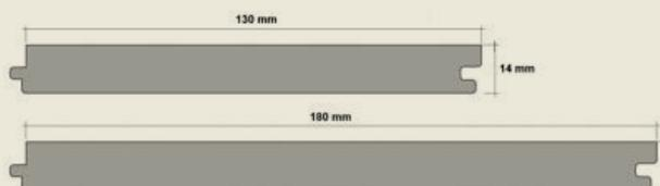
This gives the floor an equivalent wear layer to thicker flooring products and also increases the stability of the floor when under pressure from expansion. (see diagram below).
